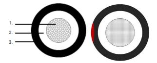
1. Conductor: Fine wire strands of non-porous tinned copper wires according to IEC 60228, Class 5
